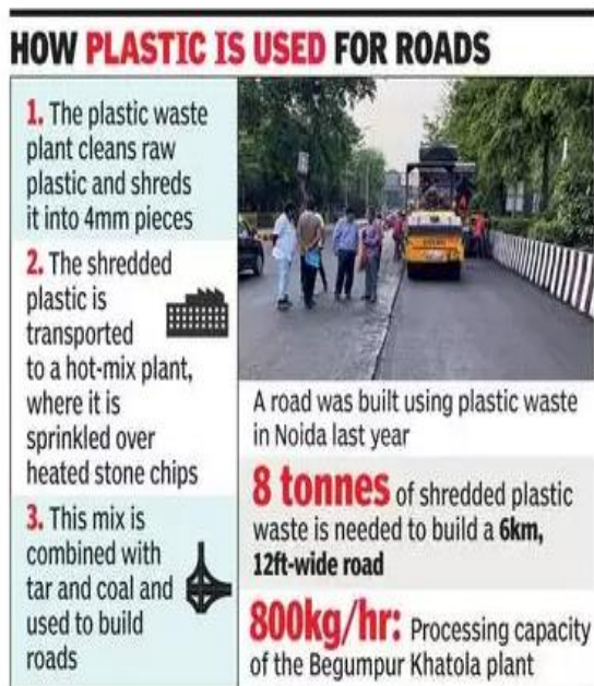
Figure 3: Use of plastic in road construction
