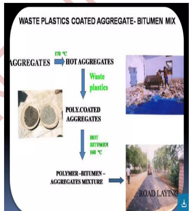
Figure 4: Overall process of using Bitumin mix for road construction
